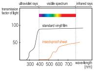
Insect-Control Sheet which prevents insects flying inside by cutting wave length of light which induces them is suitable for the food factories  $\frac{1}{2} \int_{-\infty}^{\infty} \frac{1}{2} \left( \frac{1}{2} \int_$
